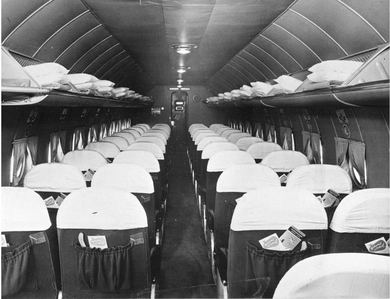
The Douglas DC-3 was wider than the DC-2, allowing 1x2 seating rows. This picture shows the Douglas DC-4 cabin, wide enough for 2x2 seating rows. Note the overhead shelving full of blankets and pillows.
