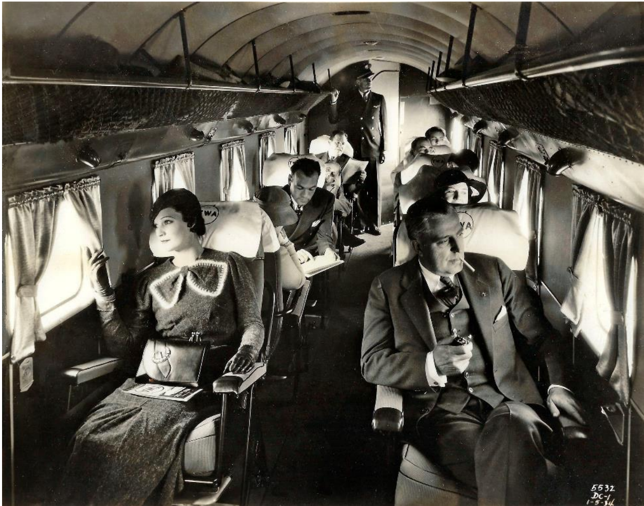
The Douglas DC-2 cabin, built to resemble railroad Pullman Coach cars. The fuselage was only wide enough for 1x1 seating with a central aisle. Notice the open overhead racks for coats, hats, and handbags. You don't have to wait until after landing to experience contents shifting in turbulence.
