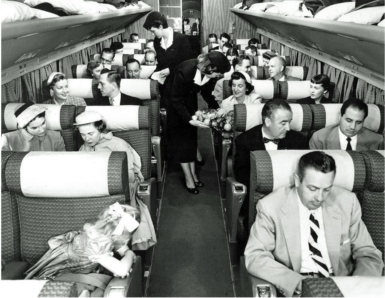
The Douglas DC-7 was pressurized and significantly faster than the DC-4, thanks to over-stressed R-3350 turbocompound engines, but the cabin was still just 2x2 seats wide. Overhead storage hasn't changed much.
